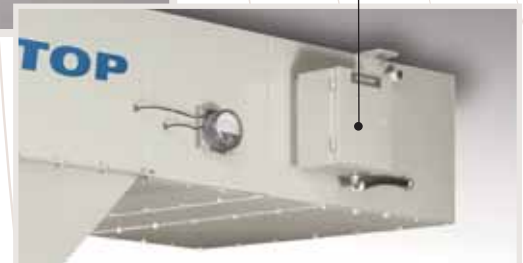
Automatic pulse cleaning control panel
